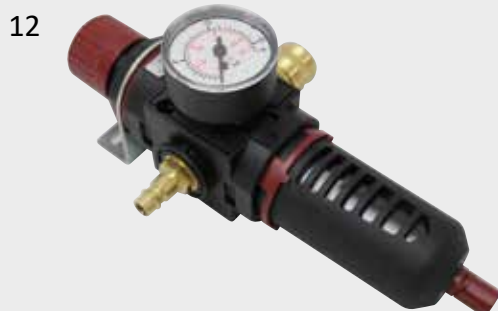
Filter regulator G3/8 with filter-pressure regulator, manometer, plastic protective cage, fastening angle, plug connection G3/8 and coupling.
