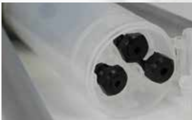
Replacement nose pieces in locked box (integrated) in the mandrel container.
