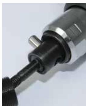
Quick change system for the mandrel.
