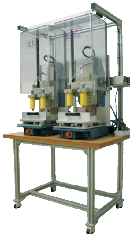
KVT Basic 5000 DUO thermal installation machine for simultaneous thermal installation of four inserts into two covers of car outside mirrors
