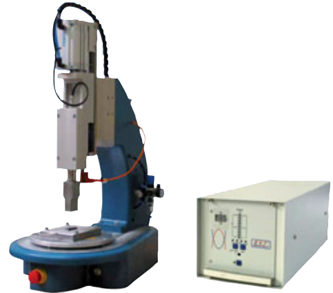
Ultrasonic welding machine with a working frequency of 35 kHz for ultrasonic riveting or welding or to embed UNITEC® K' in K' (plastic in plastic) inserts.
